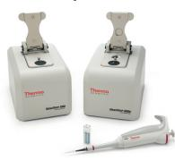
Using the patented Thermo Scientific NanoDrop<sup>™</sup> microvolume sampling technology, a 1  $\mu$ L sample can be measured in less than 5 seconds. Students simply pipette a 1  $\mu$ L sample directly onto the pedestal, measure and wipe clean. In addition to the pedestal, the NanoDrop 2000c instrument offers a cuvette position for larger volumes.
